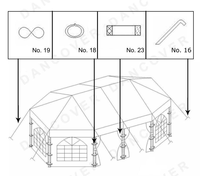
**Step 12:** Put the corner draperiens on the tent using the rings **Step 13**: Secure the tent with guy lines (No. 19) and stake pegs (No. 16) as shown above.
