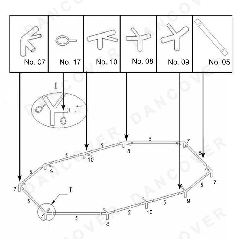
Step 1: Lay out the basic shape as shown above.
