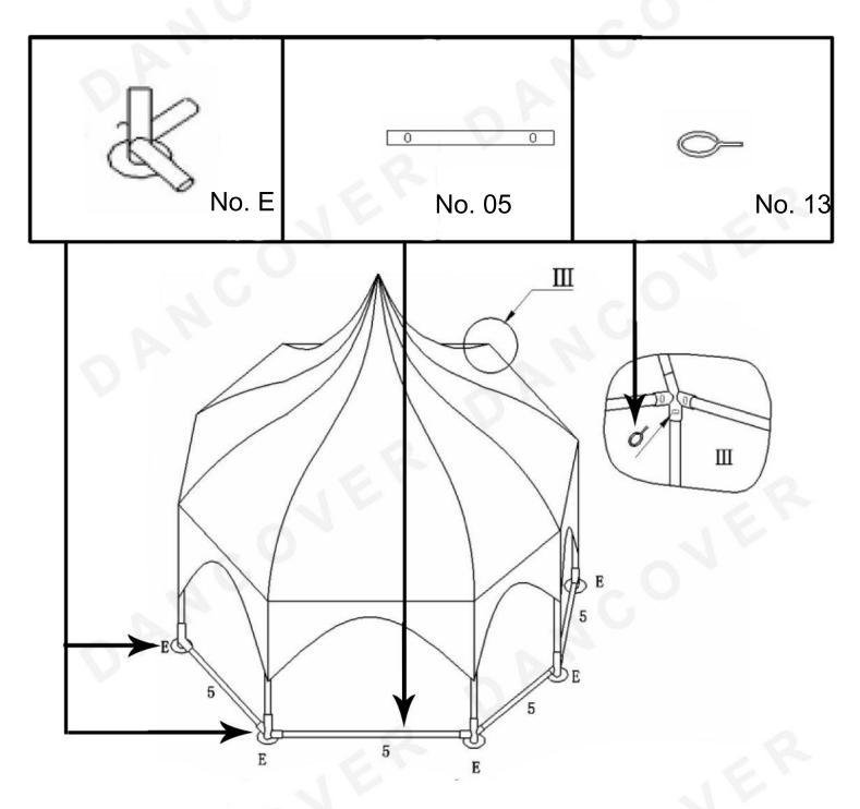
**Step 7:** Secure the legs to the roof structure as shown in III. **Step 8:** Place the feet (no. E) on the structure an connect them with theground bars (No. 05).
