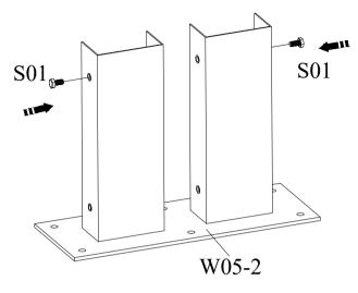
Pre-install 2pcs S01, as height position for burying part under ground.
